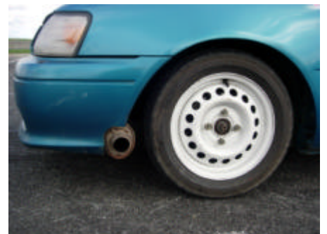
Piers MacFheorais's claims his cunning exhaust system (yes, that is the front wheel) not only saves weight but also gives the car a more favourable weight distribution
