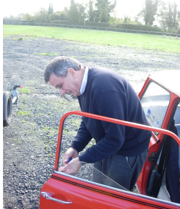
Myles O'Reilly takes a break from his stewarding duties to remove the windows from Philip's Mini – a very sophisticated two self-tapper arrangement holds them in position
