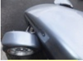
Darren Quille's Westfield has sculpted mudguards to cope with its enhanced turning circle
